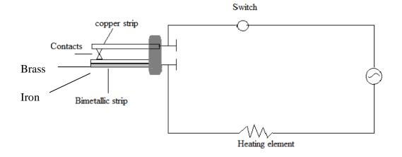
17) The figure below shows a circuit diagram of a device for controlling the temperature in a room.
