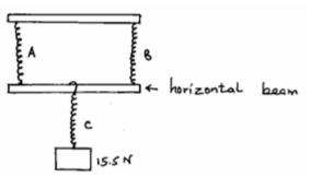
If the weight of the horizontal beam is 0.5N, determine the extension of each spring given that 4N cause an extension of 1cm when using one spring. (3mks)
