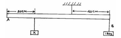
The rule is 1m long and weighs 1.8N. Calculate the weight of the block X. (3mks)
