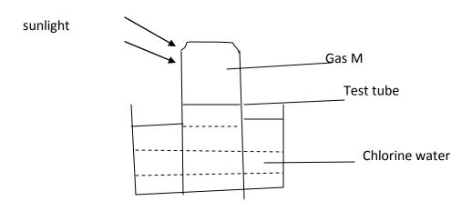
After one day, a gas M was found to have collected in the test tube as shown above.
