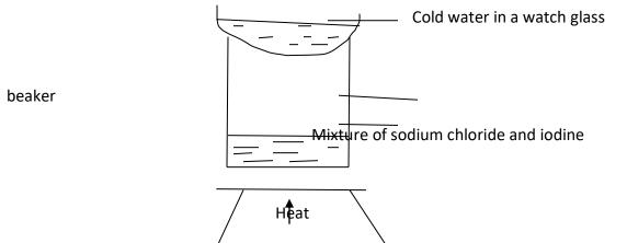
(a). the mixture was heated for some time and left to cool. On cooling, shiny black crystals and white crystals were observed on the surface of the watch glass and in the beaker respectively. Name:
