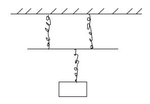
Given that one such spring extends by 2cm when a load of 20N hangs on its lower end, determine total extension of the system. (3mks)
