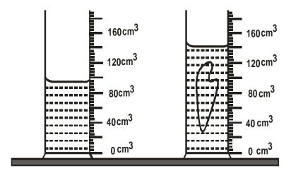
Given that the mass of the solid is 268g, determine the density of the solid in SI units.
