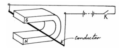
(a) Indicate on the same diagram the direction in which the conductor swings when the switch K is closed. (1 mark)
