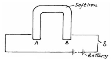
Complete the circuit by drawing the windings on the two arms of the core so that A and B are both north poles when the switch S is closed. Indicate the direction of the current of the windings drawn. (1 mark)
