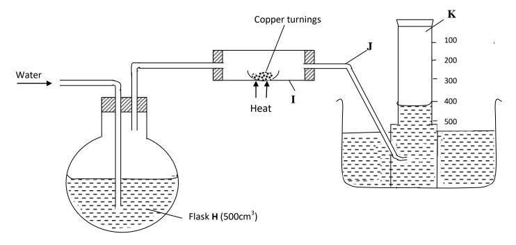
A 500cm<sup>3</sup> measuring cylinder **K** was filled with water and assembled for gas collection. Copper turnings were heated red hot and water was slowly passed into 500cm<sup>3</sup> flask **H** until it reached the 500cm<sup>3</sup> mark. A colourless gas was collected in **K**.
