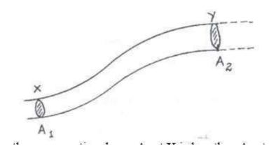
If the cross-sectional area A1 at X is less than A2 at Y, state how the liquid velocity V2 at Y
