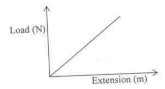
On the same axes sketch a graph for a spring double the diameter and half the length of the first one.
