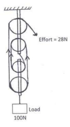
If the effort applied is 28N and the load lifted is 100N, determine the efficiency of the system
