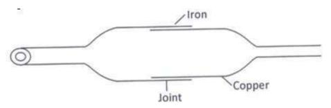
Explain how you would separate the two by changing the temperature given that copper expands
