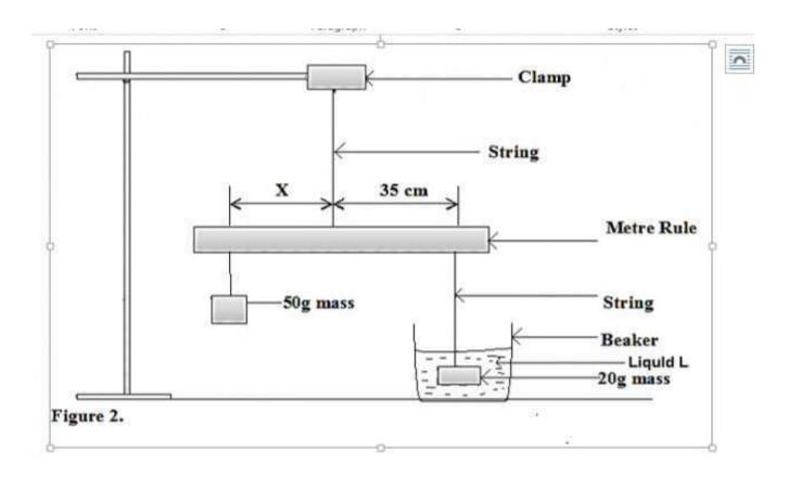
Lower the 20g mass until it is completely immersed into liquid L provided in a beaker and adjust the position of the 50g mass until the metre rule balances horizontally. Read and record X, the distance of the 50g mass from the centre of gravity of the metre rule when the rule balances horizontally.
