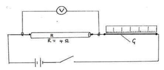
i)Use the voltmeter provided to measure and record VR, the potential difference (pd) across R and the Vg, the Potential difference across G when the switch is closed.
