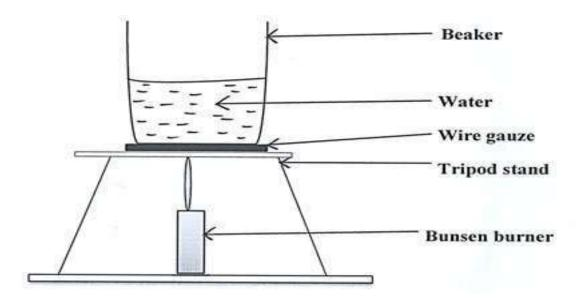
Using the measuring cylinder, measure 100cm3 of water and put it into the beaker. Take the initial temperature, T0 of the water.
