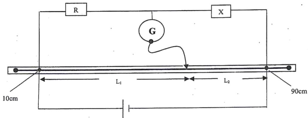
(i) Move the Sliding pointer along the resistance Wire until the galvanometer reading comes to Zero. Record  $L_1$  and  $L_2$ .
