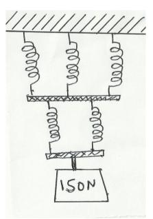
Determine the total extension caused by the 150N weight.
